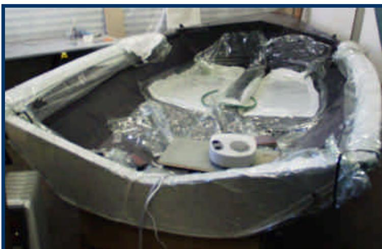
Photo 20 (above) the decks and transom being laminated and vacuum bagged
