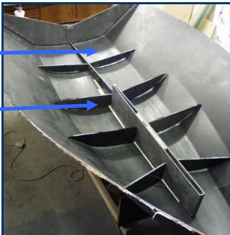
Photo 11 (above) shows a typical bulkhead layout using a combination of perpendicular and angled bulkheads. Angled bulkheads produce a stiffer boat but it is harder to shape the pieces to fit.
