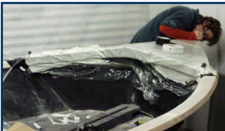
Photo 19 (above) the foredeck being laminated and vacuum bagged
