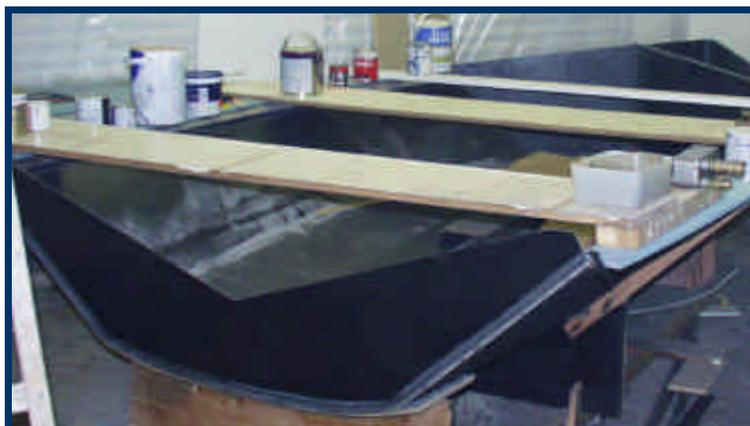
Photo 16 (above) side deck foam being bonded in place
