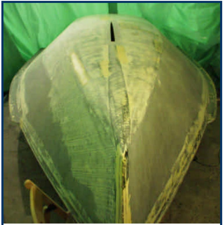
Photo 22 (above) shows the hull after a layer of filler has been scraped over the whole surface
