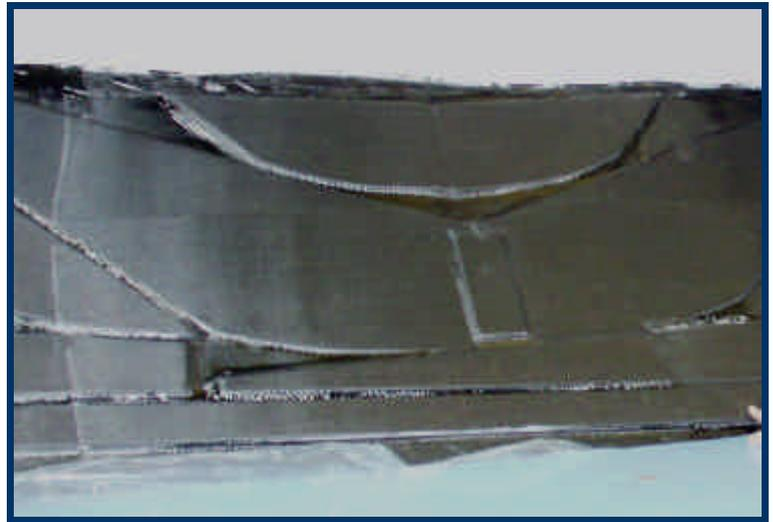
Photo 6 above shows the transom and the central spine component being laminated. The components have been cut to size and fit checked by offering up to the hull before laminating
