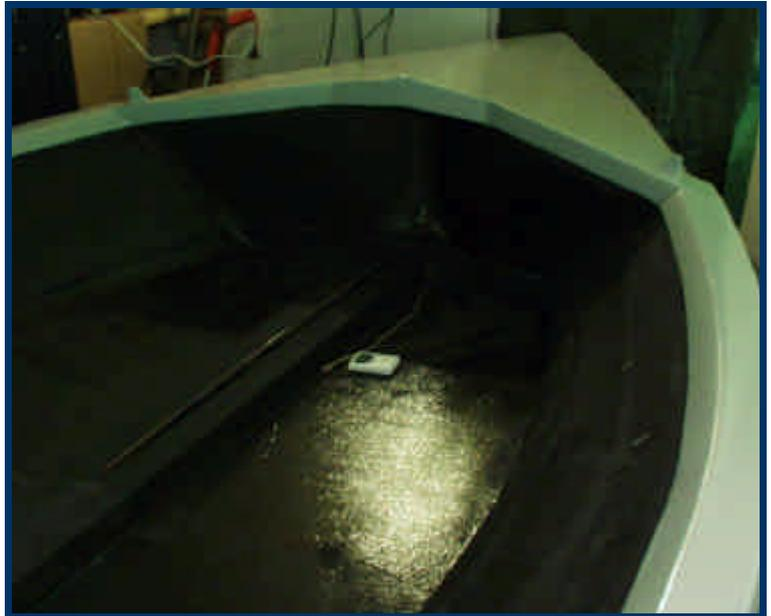
Photo 21 (above) Hybuild applied to the decks,
