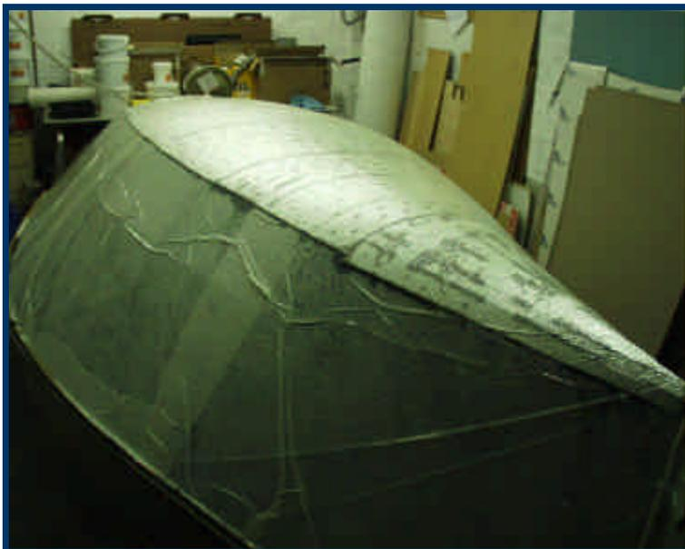
Photo 1 (above): Hull inner skin being vacuum bagged
